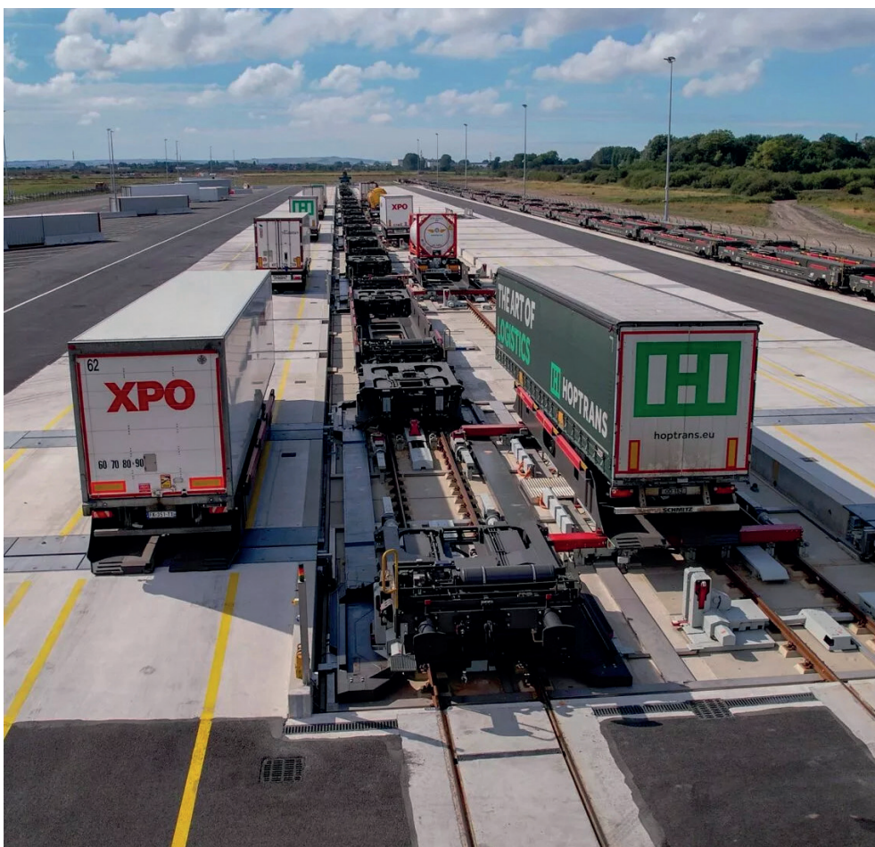
CargoBeamer has developed technology to support the movement of non-craneable lorry semi-trailers by rail.
