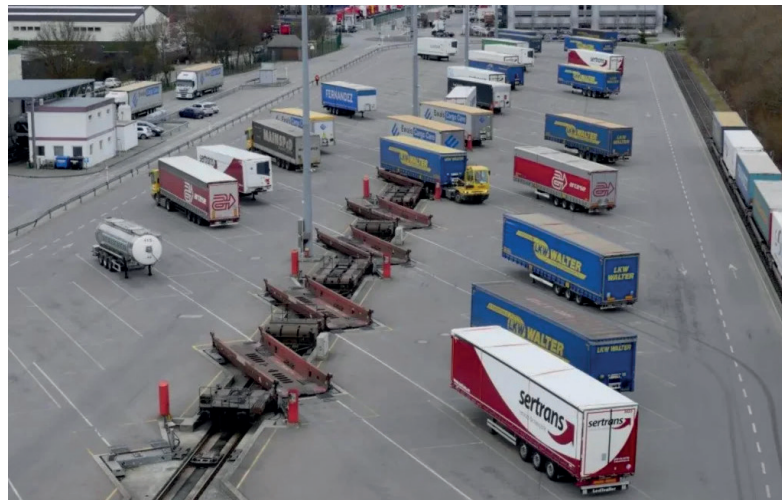
Loading semi-trailers onto Modalohr wagons at a dedicated terminal.
