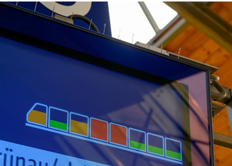
[14] Real-time information: Pilot project for the occupancy of S-Bahn cars at the S-Bahn Berlin. The occupancy rate is measured with a light sensor and displayed in real time
